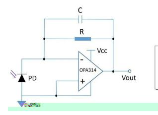
$V_{out}(V) = I_{ph}(A) \times R(\Omega)$
