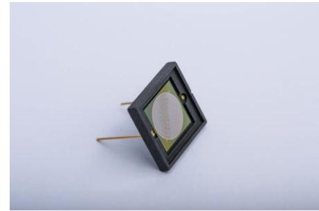
**Applications:** EUV radiation monitoring and flux measurement
